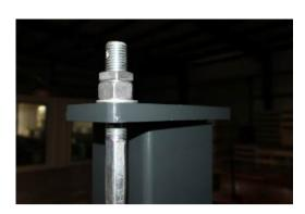
• With the cables routed through the ramp and posts, secure them to the post caps with the nuts provided.
