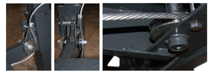
• With the ramps installed on the cross beams, be sure cable routing matches the images above, and that the cables are fully seated in the pulleys.
