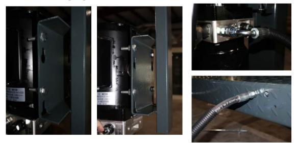
• With the locking mechanism installed, proceed to install the hydraulic pump, and connect the hydraulic hose from the pump to the ramp.
