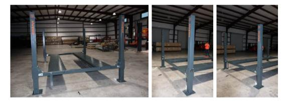
• With the posts spaced accordingly, place the platforms on the cross beams, and secure with the bolts provided.
